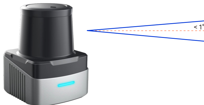
Figure 6. Schematic diagram of the vertical laser angle
